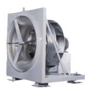
The standard Air Handling Unit Fan Section contains a double inlet double width fan with either multiblade forward curved, backward curved or backward curved areofoil bladed implellers. Alternative fans are available.
